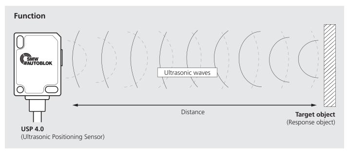
The **USP 4.0 Ultrasonic Positioning Sensor** measures the distance to objects without contact. The sensor emits ultrasonic waves. If these hit an object, they are reflected. The resulting echo is picked up by the sensor and the distance to the object is calculated from the time between the transmission and reception of the sound pulse.
