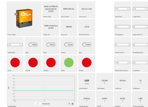
The gripper can now be controlled by toggling the control bits or changing parameters
